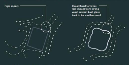
Hong Kong is prone to severe weather conditions such as tropical storms and typhoons that can damage buildings. **The Henderson** employs a hi-tech, 4-ply, double-curved, double insulated glass facade to withstand the powerful typhoons that impact buildings. The facade design offers maximum visibility of outdoor views whilst UV rays are blocked and the building interior is insulated against Hong Kong's summer heat.
