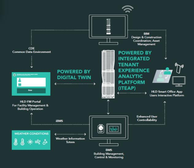
Digital Twin an integrated platform for building operation, user engagement, openBIM and GIS, asset management, ESG performance, carbon assessment, throughout the building life
